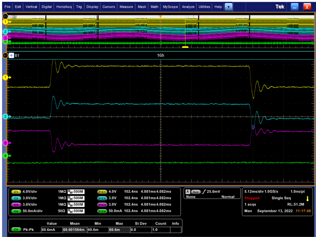
Figure 159: Ignition without capacitor (segment A2825) (2)
