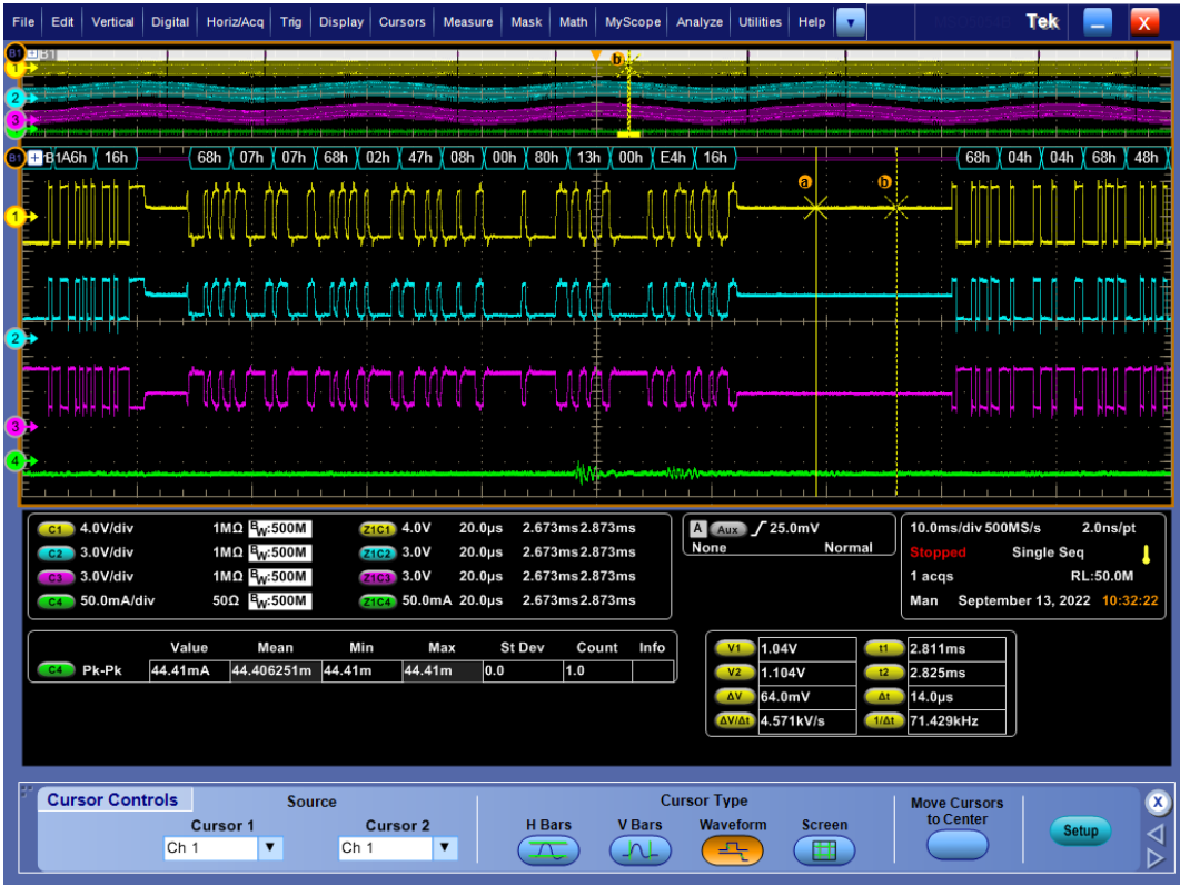
Figure 150: Zero measurement with loose capacitor no burner pulses (segment A2825) (2)
