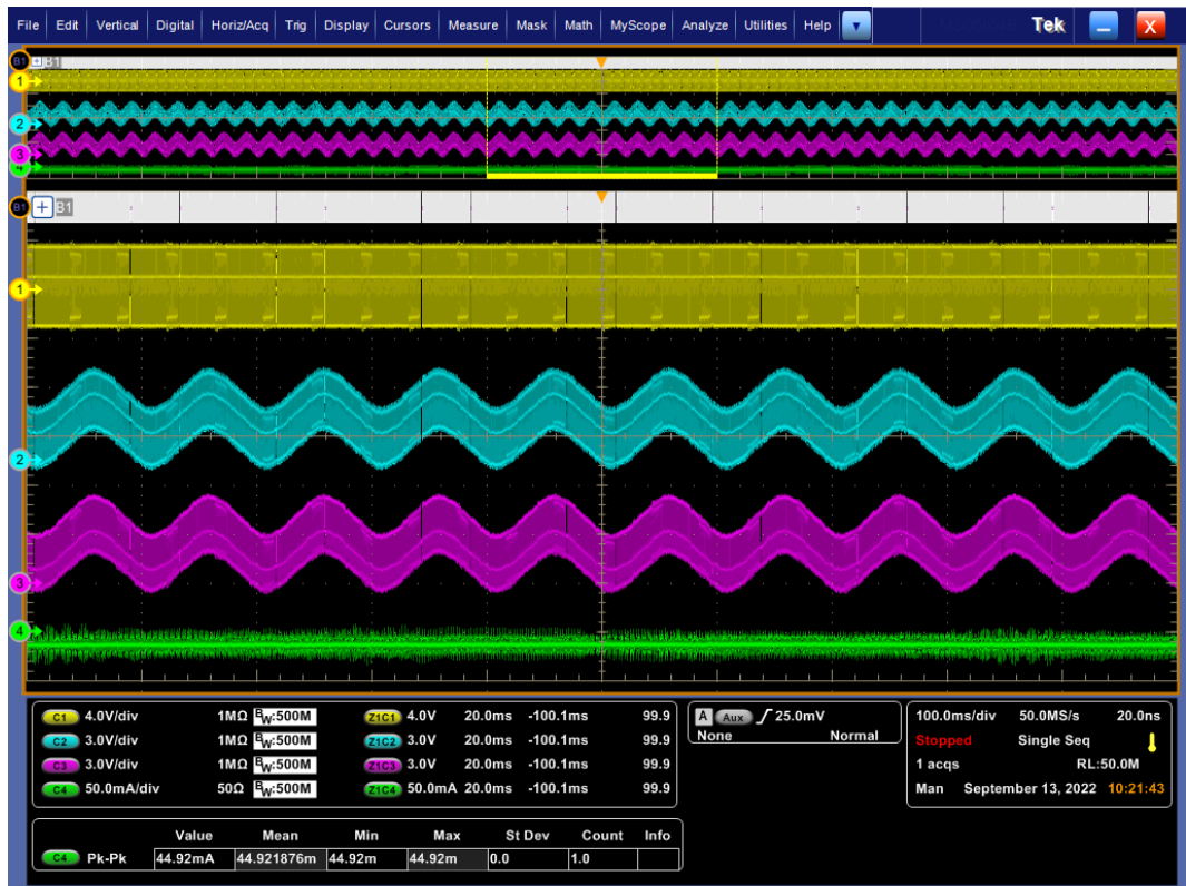
Figure 149: Zero measurement with loose capacitor no burner pulses (segment A2825) (1)
