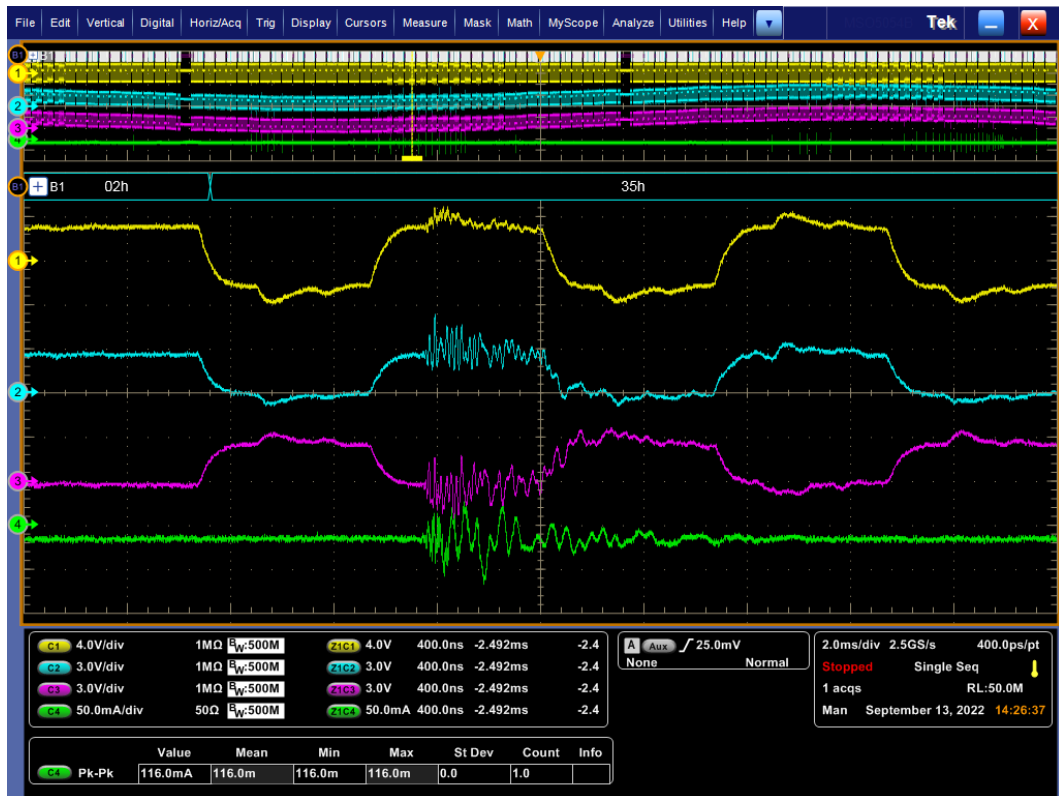
Figure 175: Ignitions only on other segment (A2823) with Würth Elektronik DB9 with capacitor and wire on spark plug (2)
