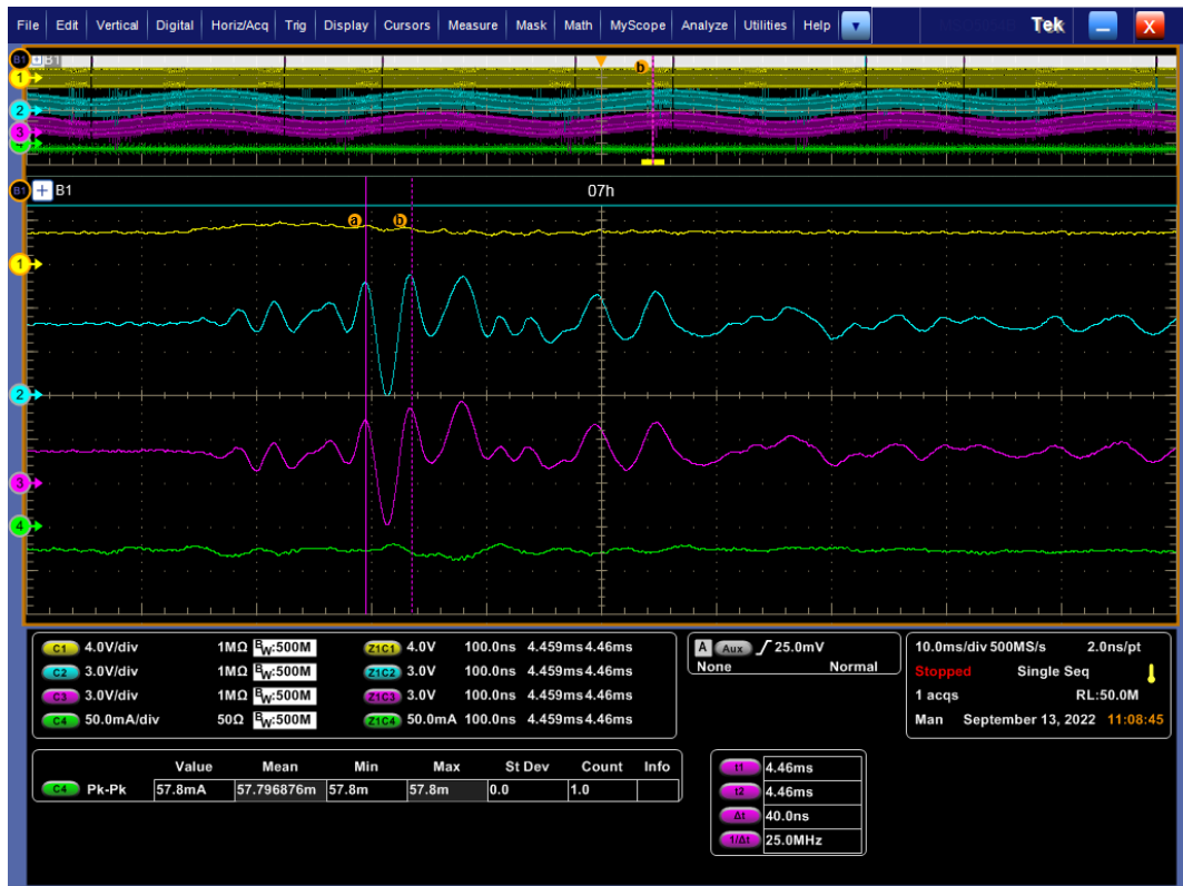
Figure 156: Ignitions with separate capacitor (segment A2825) (3)
