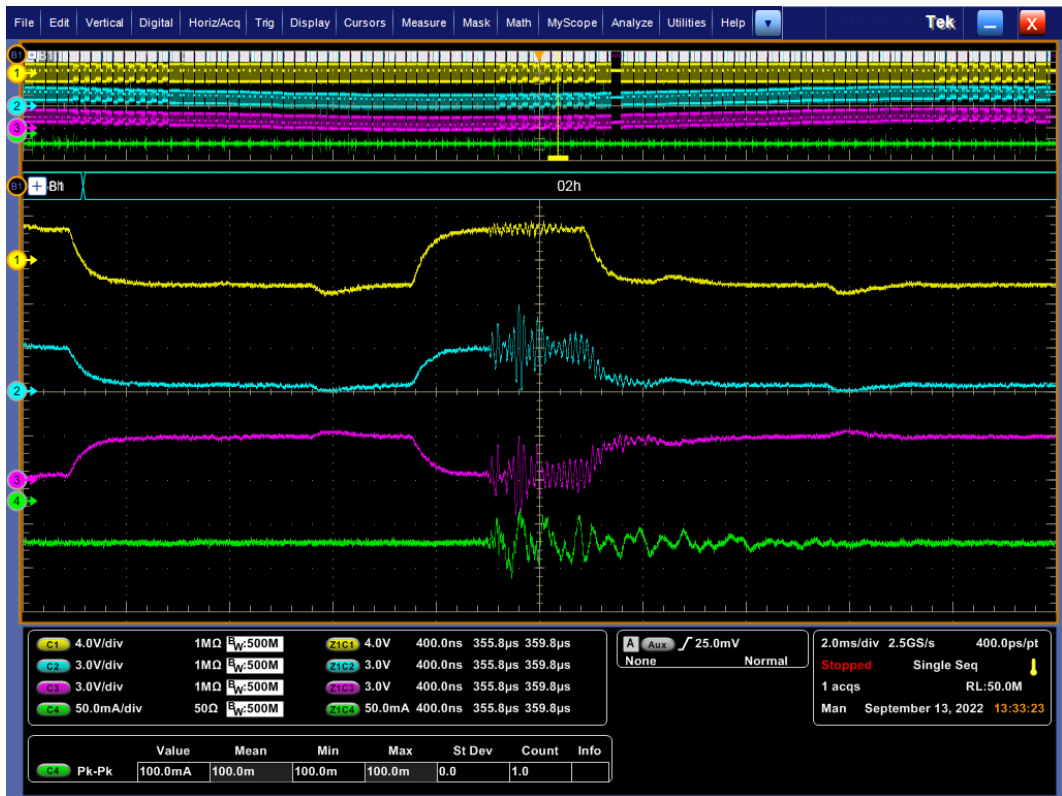
Figure 164: Ignitions on another segment (A2823) with Würth Elektronik DB9 with capacitor (measurement on segment A2825) (3)
