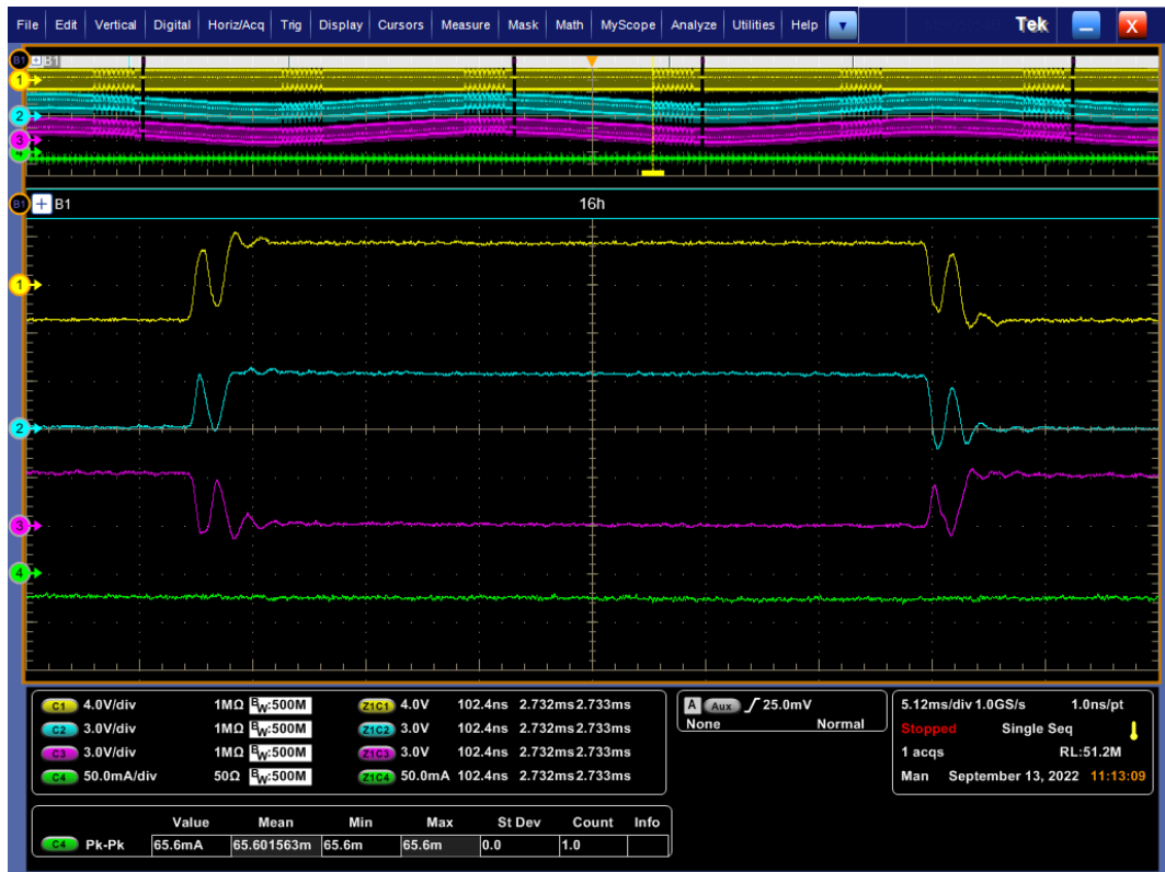
Figure 157: Ignitions with separate capacitor (segment A2825) (4)
