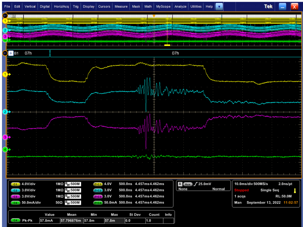
Figure 155: Ignitions with separate capacitor (segment A2825) (2)
