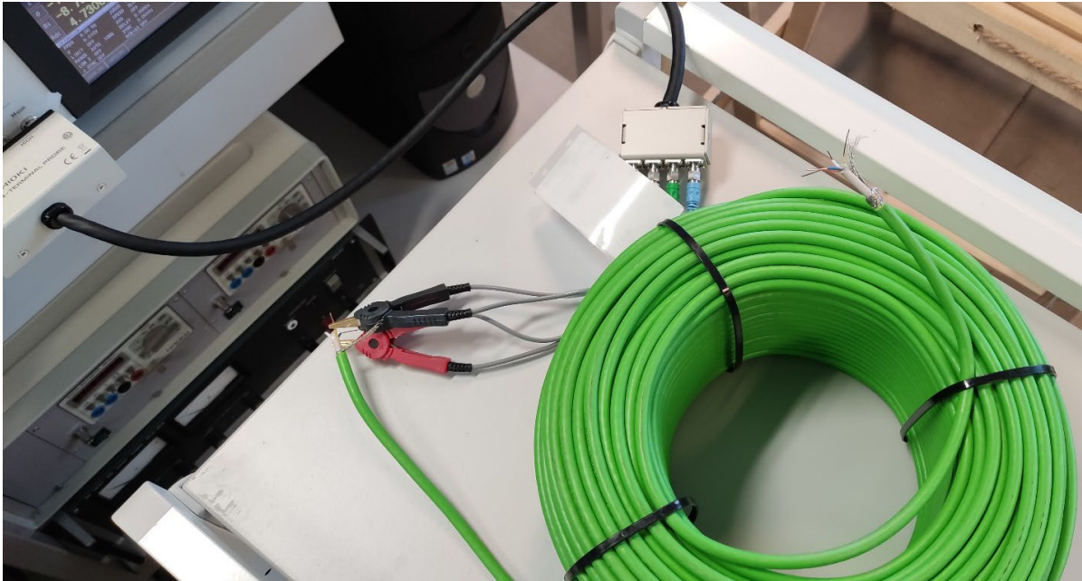
Figure 46. Rolled cable under test (OC measurement).
