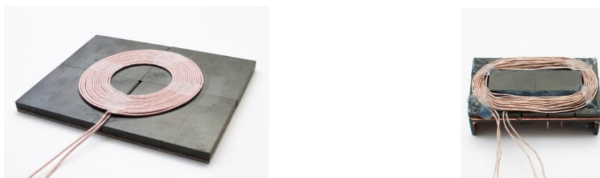
Figure 6 Initial Litz wire coils for wireless mouse charger, left: transmitter, right: receiver
