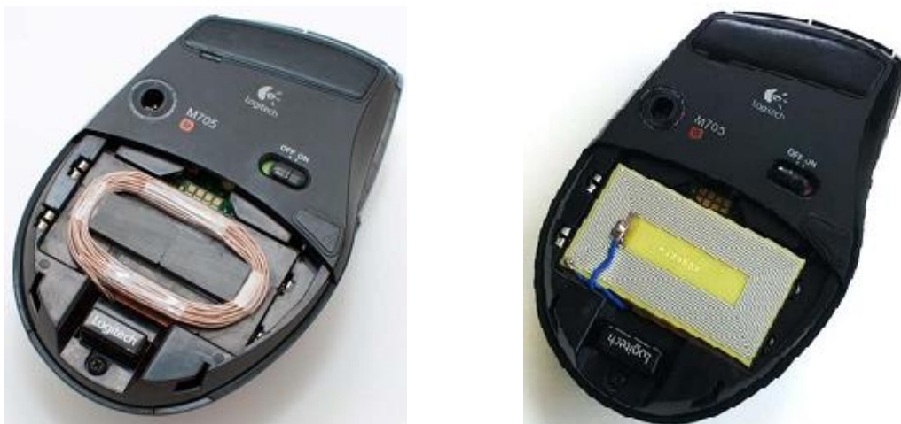
Figure 5 Wireless mouse test case with receiver coil using different technologies, left: Litz wire, right: PCB
